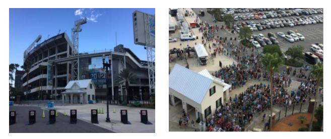
As shown in the photos above, these barriers allow for foot traffic flow, however, will not allow a vehicle to enter the area for a possible ramming incident. These barriers are portable so they can be moved to events as needed throughout the region. Florida is in the process of purchasing additional barriers to be used in other areas across the state.
