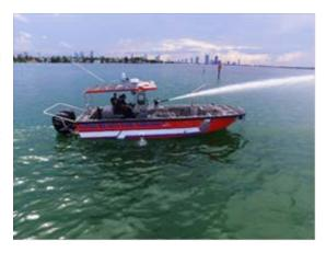
the water; a 1000 GPM fire pump that draws sea water through a built in sea chest; and removable doors with a dive ladder on either side to make water rescues more efficient.
