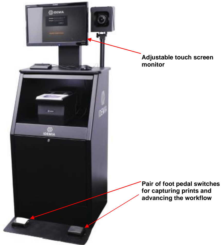
Figure 12: Fixed-Height Cabinet's Pedal Switch for Capturing Prints.
