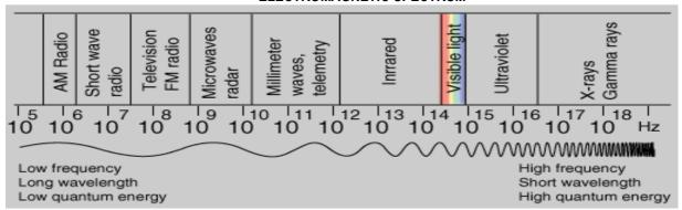
A wavelength is the distance between one location of a wave of light such as a peak or crest and the next corresponding location.
