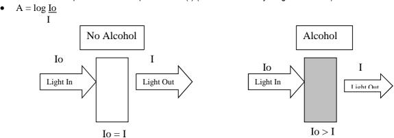
• The more alcohol molecules there are in the sample, the more light will be absorbed by these molecules, the less light will reach the detector and the higher the alcohol result will be.
